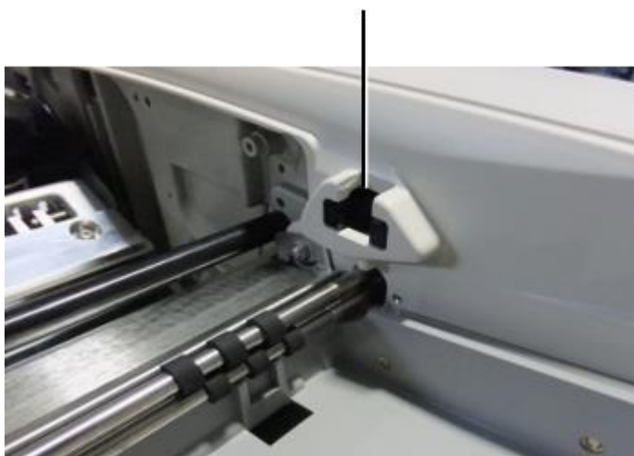
Top cover closed sensor
